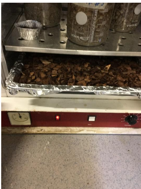
Figure 29. Drying oven, capable of maintaining a temperature (100 °C), pine bark sample
