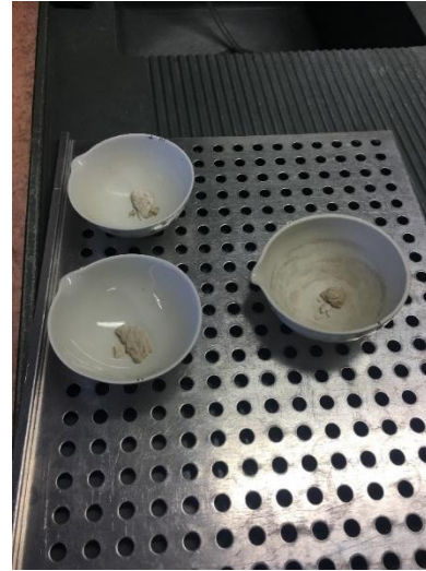
Figure 30. a) Samples prepared for control burning, b) after process of burning
