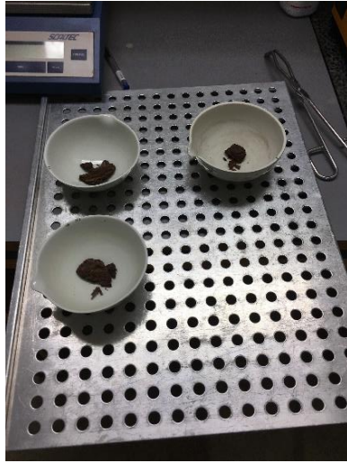
Figure 30. a) Samples prepared for control burning, b) after process of burning
