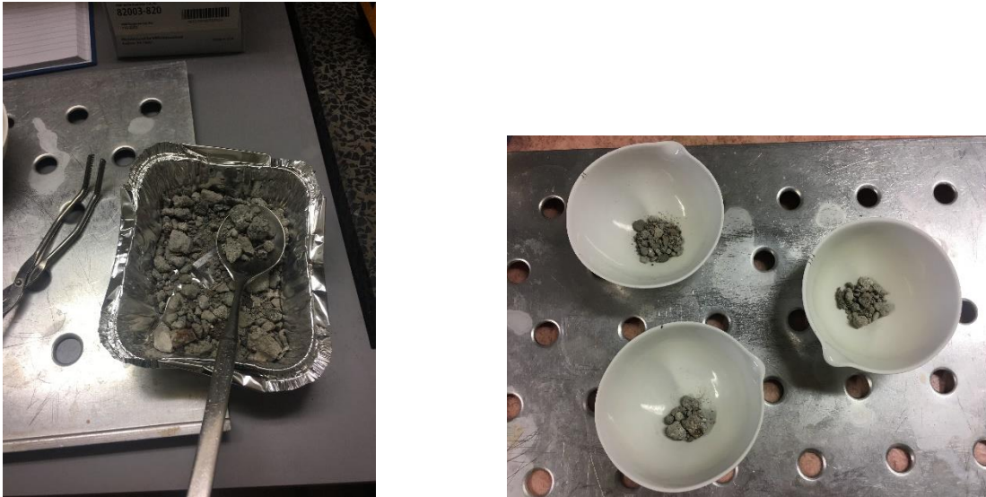
Figure 28. Samples after drying and burning process, respectively
