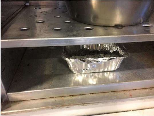
Figure 26. Drying oven, capable of maintaining a temperature (100 °C), bottom ash sample
