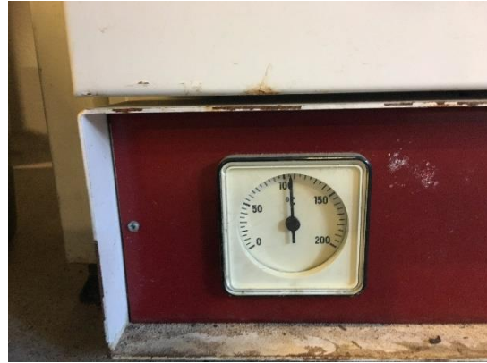
Figure 26. Drying oven, capable of maintaining a temperature (100 °C), bottom ash sample
