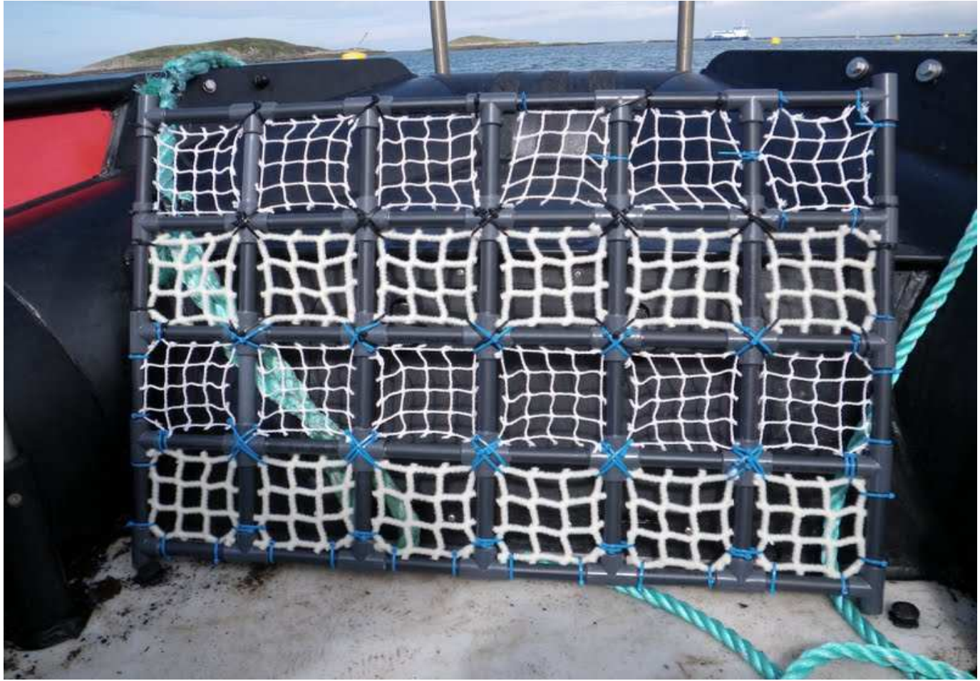
Figure 8: PVC frame with nylon and Micanti samples mounted on with cable ties (Photo by Pudota).
