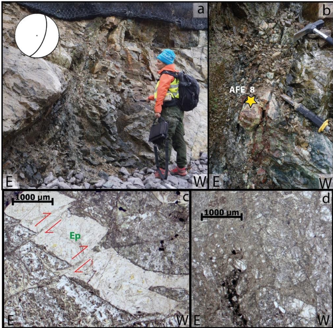
Fig. 4-14: Bjånes Fault Zone 6, Cataclastic fault. (a) Overview of the fault with a high strain zone to the east and an ambiguous contact towards the west to the fresh, undeformed anorthosite. (b) Zooming into the cataclastic fault core. Note the various mineral phases in band parallel to the fault core. (c) Vein filled with Ep investigated in the microscope. Microfaults indicate a dextral sense of shear. (d) Cataclastic deformation dominates towards the east.
