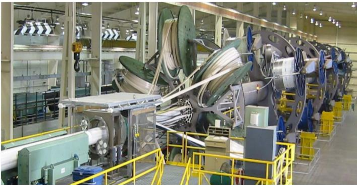
Figure 2.4: Closing machine (horizontal), [6]
