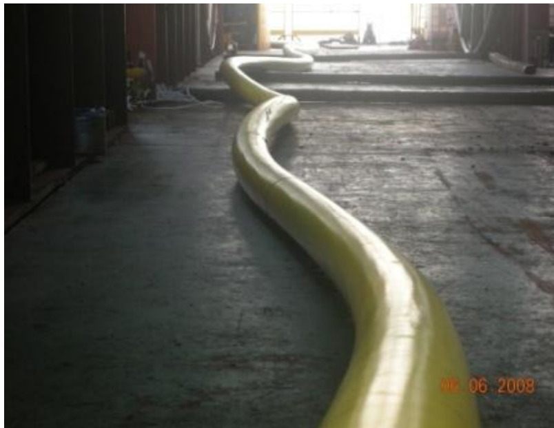
Figure 1.1: Snakelike configuration in a deformed umbilical.
