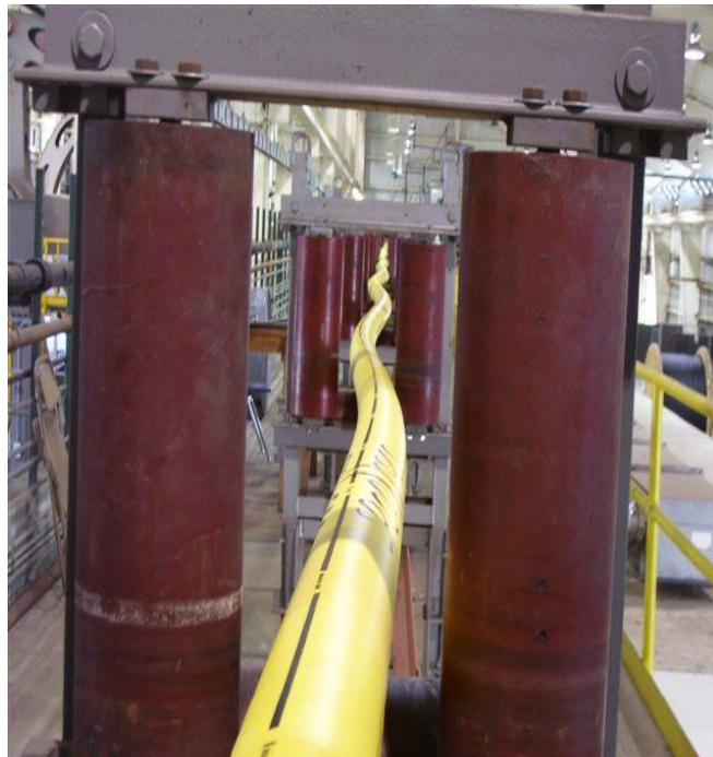
Figure 5.5: Snakelike deformation of Droshky
