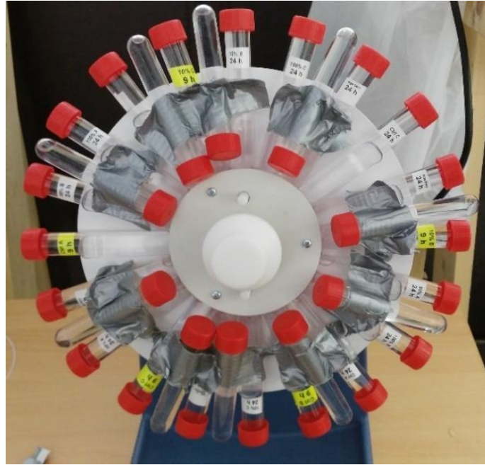
Figure 2.2. The rotating wheel with the vials wit algae solution was spinning at 2 rps to keep the cells from settling, and kept at the selected temperature.
