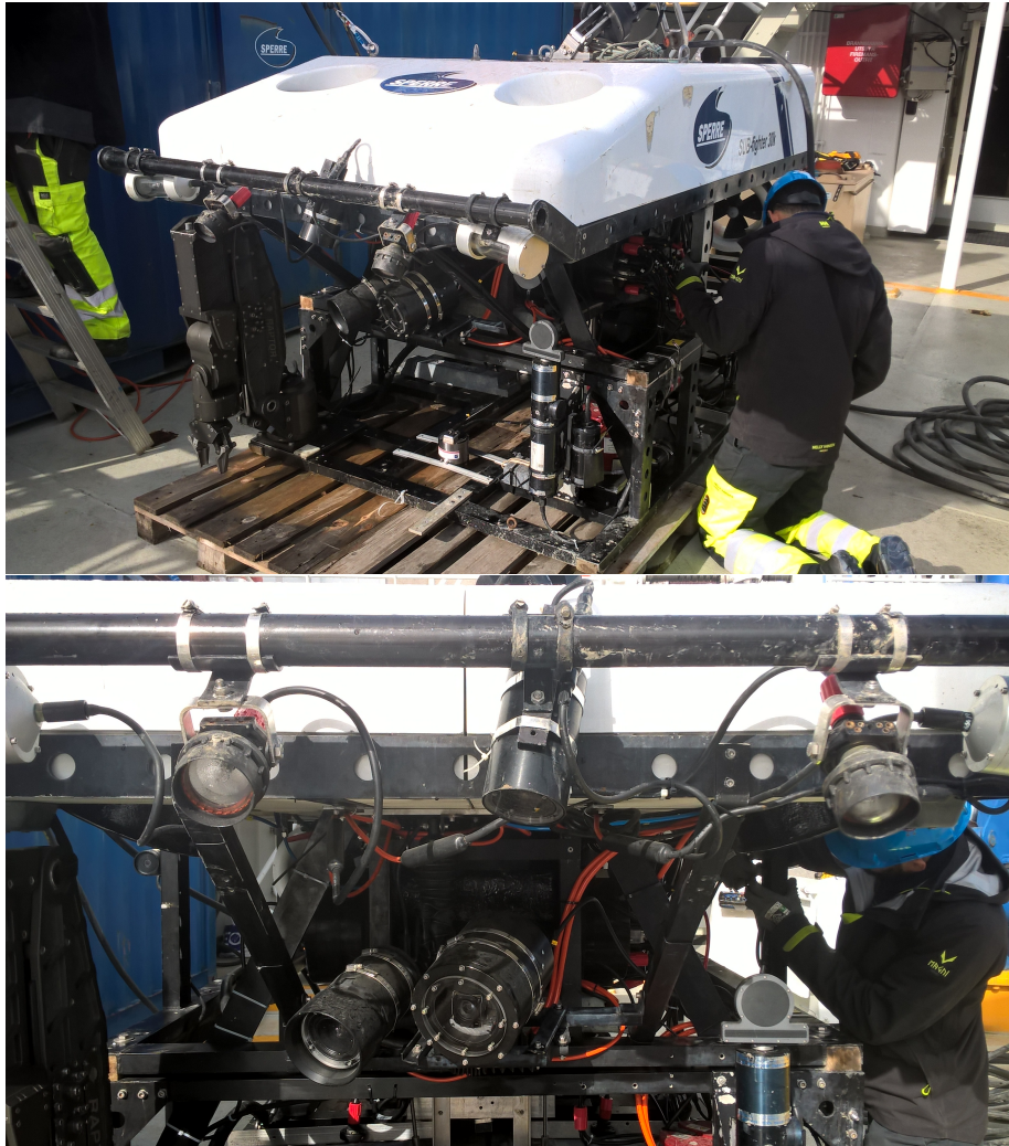
Figure 4: ROV Sperre. The first image shows the Sperre sub-fighter 30k ROV. The second image shows affixed lamps and cameras.
