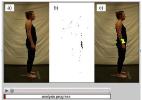
**Figure 4.** Screenshot of the video software. a) Input video; b) Motion image. (pixels in white indicate no movement occurred between the frames, and pixels in black represent movement) c) Illustration of the displacement of the centroid of motion.
