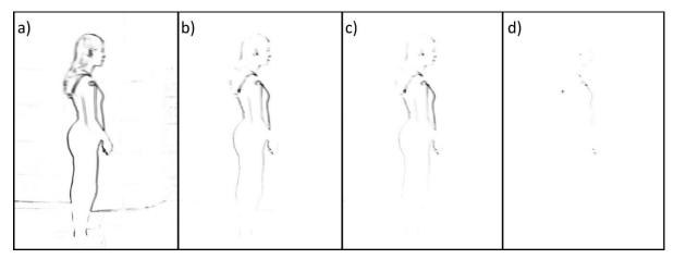
**Figure 5.** Illustration of four different filter settings in the motion image. a) 0,01; b) 0,02. (the one chosen) We chose the filter setting 0,02 due to apparently little noise and detection of real movements in the participants; c) 0,03; d) 0,05.
