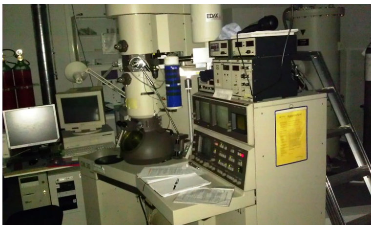
Figure 3.12: Picture of the CM30 used. The column, with the screen below, is left to the blue thermos.
