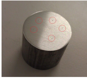
Figure 3.4: Picture of one sample with indentations made by the hardness tester.
