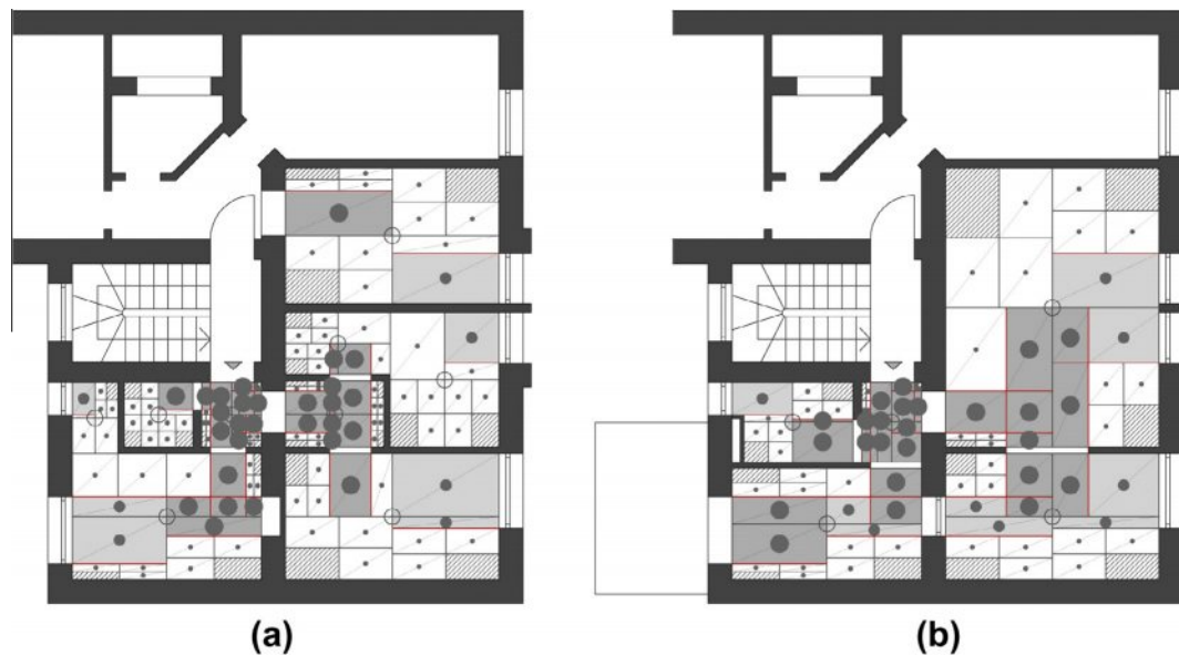
Figure 3. Placement of perceptual centres: Plans of the first floor before (a) and after (b) the dwelling renovation. Residential building, Cologne, Germany. © [detail]. Reproduced by permission of detail.
