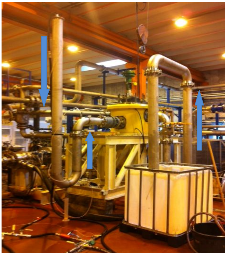
Figure 9: Multiphase pump arrangement from experiments
