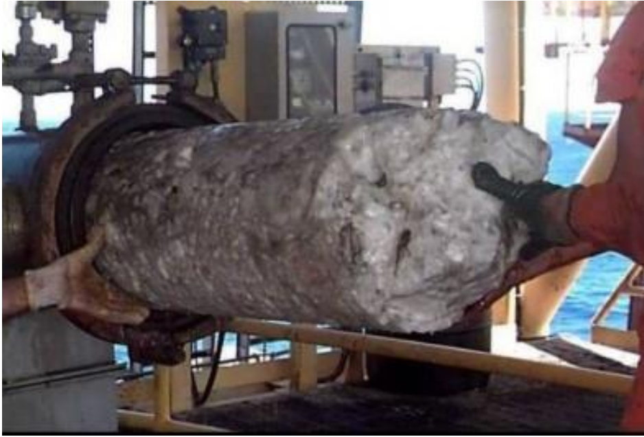
Figure 1: Hydrate plug removal
