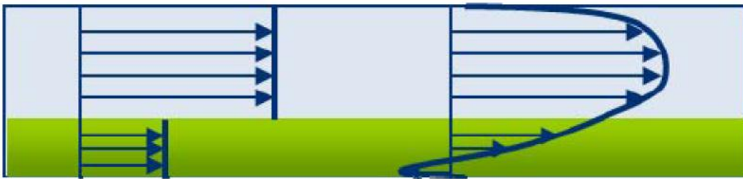
Figure 3 Velocity profile: 1D to the left and Q3D to the right
