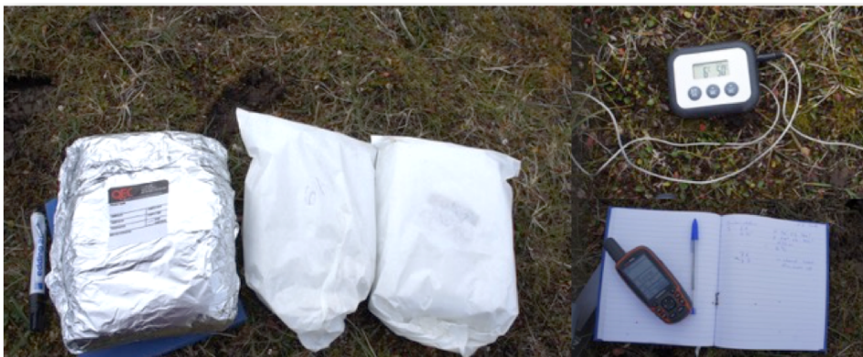
Figure 3.2: Samples were wrapped in aluminum foil and labeled (left). On the right, soil temperature in comparison to the air temperature and GPS coordinates and attitude were determined.
