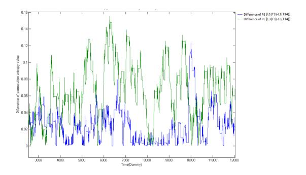
Figure 4: Difference of permutation entropy values of  $L_1$  and  $L_3$  waveforms for turbines 3 and 14.
