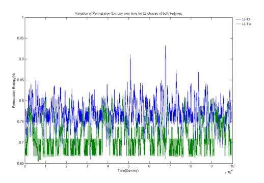
Figure 3: Comparison of permutation entropy values for  $L_3$  min waveforms of both turbine 3 and 14.
