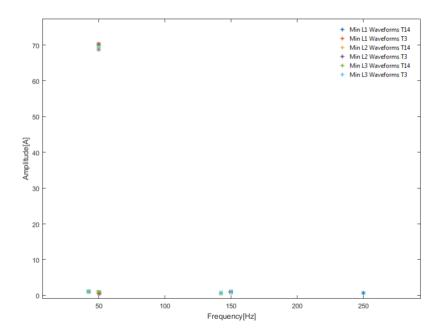
Figure 1: Amplitude vs Frequency plot for the  $L_1, L_2, L_3$  current waveforms of turbine 14 and 3
