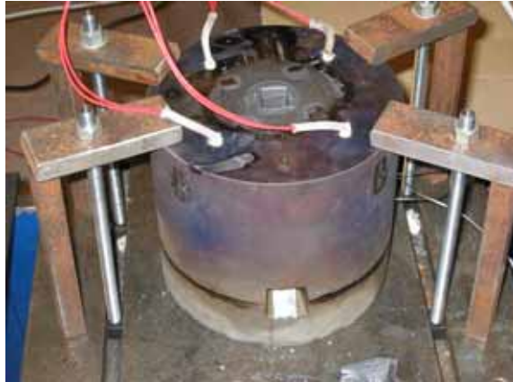
Figure 3.1: ECAP die Version 1.1 mounted on working table with the four heating elements. Entrance channel at the top and exit channel pointing towards the reader.
