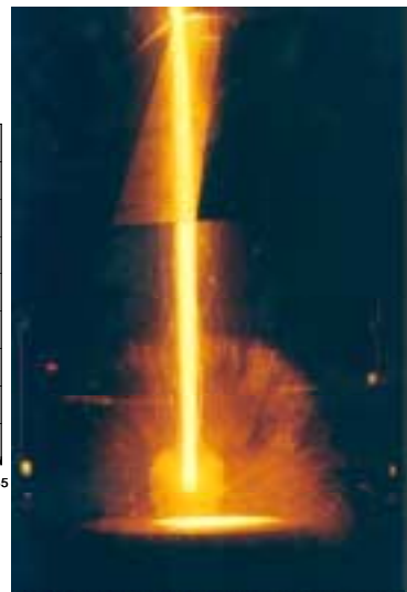
Figure 9.32 – Time-pressure trace and open-shutter photograph for a drop of Si alloyed with Al (alloy B). The drop triggered only 20 mm from the impactor ( P_{\text{trig}}=8.5 MPa).
