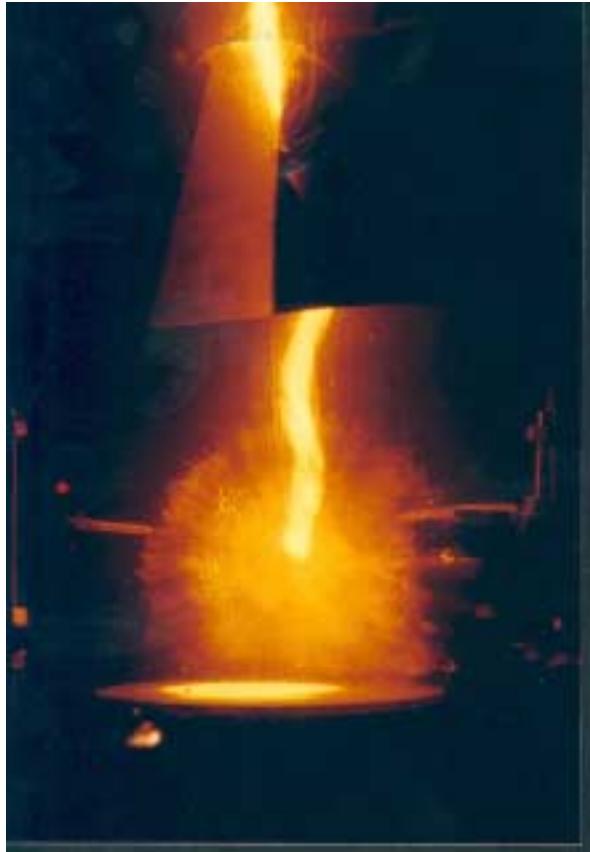
Figure 8.1 – A typical image of a steam explosion of a molten drop of silicon. Circles centered in the (estimated) middle of the bubble are drawn, and an approximate value for the bubble diameter is thus obtained.
