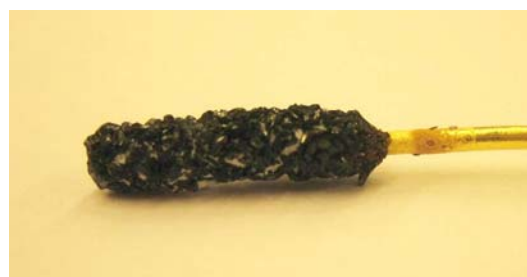
Figure 4.51 Al-Au-Na alloy deposited at 0.6 V on a gold electrode during four hours in the alumina saturated synthetic cryolite.
