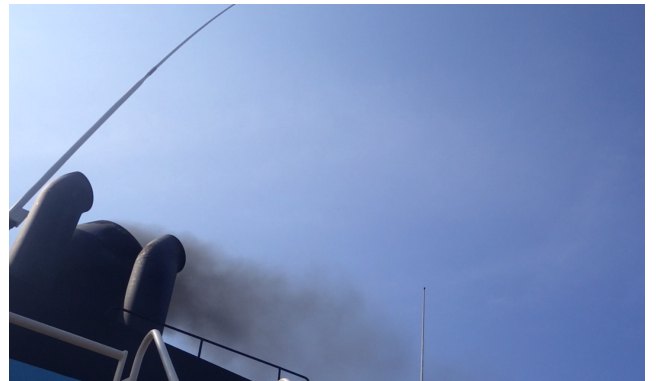
Figure 14: Exhaust smoke level with adaptive feedforward controller during engine speed step. Gray smoke is emitted for 20 seconds.
