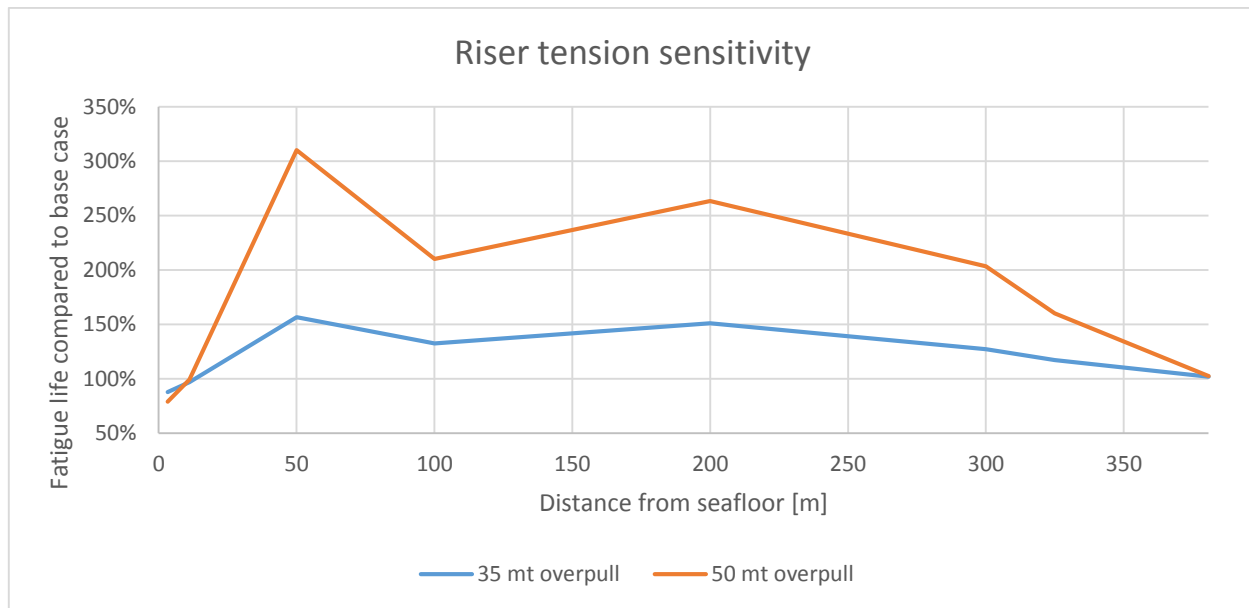
Figure 6.6: Deviations in fatigue life along the riser due to overpull variation
