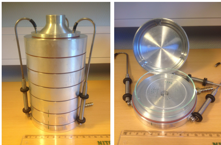
Figure 6: The Andersen sampler used to sample bioaerosols directly onto TEM grids. (a) The completely assembled Andersen sampler. The TEM grids were placed in the last stage, i.e. the bottom of the sampler. (b) The inside of the last stage. The disk in the back of the image in (b) contains a large number of 0.24 mm holes, and goes over the glass petri dish and acrylic glass plate, which contains the TEM grids. The green markings represent spots that lie directly underneath a hole.
