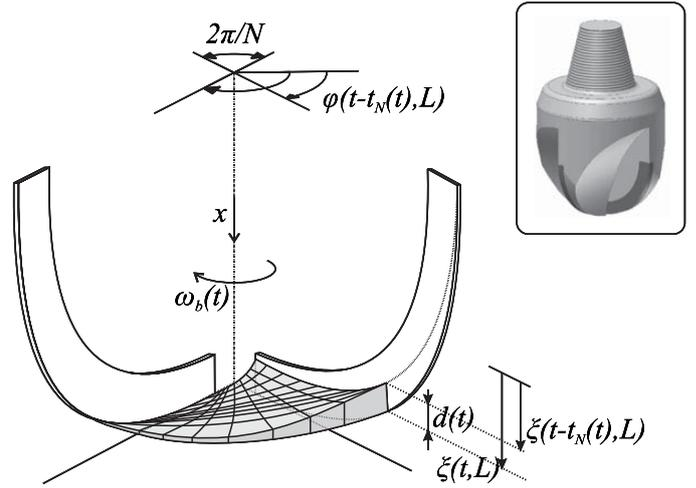
Fig. 3. Bit-rock interaction [Geramay et al., 2009].
