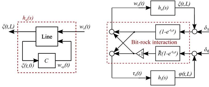
Fig. 4. Block diagram showing the regenerative effect of the Bit-rock interaction causing feedback to the drill string system [Aarsnes and Aamo, 2015].
