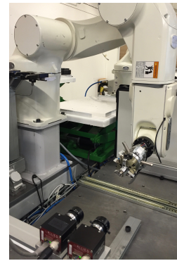
Fig. 5. Robot in the inspection pose
