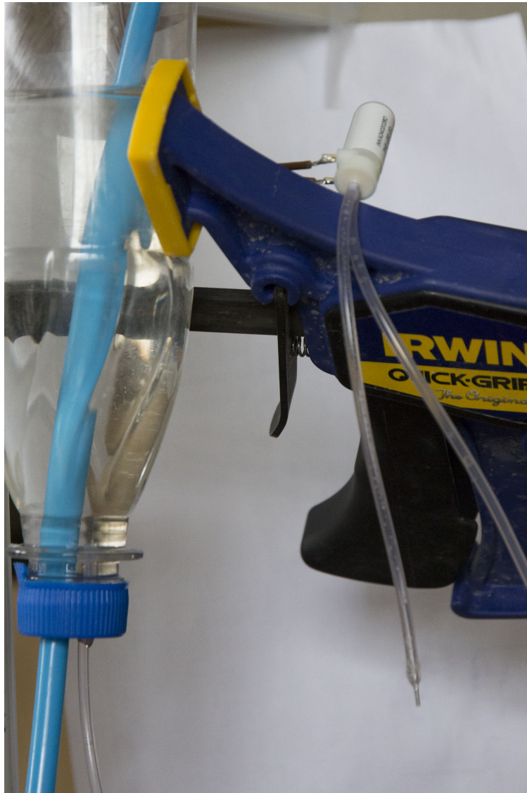
Figure 7.1: Test setup with pressurized liquid, valve and nozzle.
