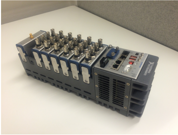
Figure 3.1: Compact RIO-9036. Here seen with 6 modules for acceleration data input and one GPS synchronization module
