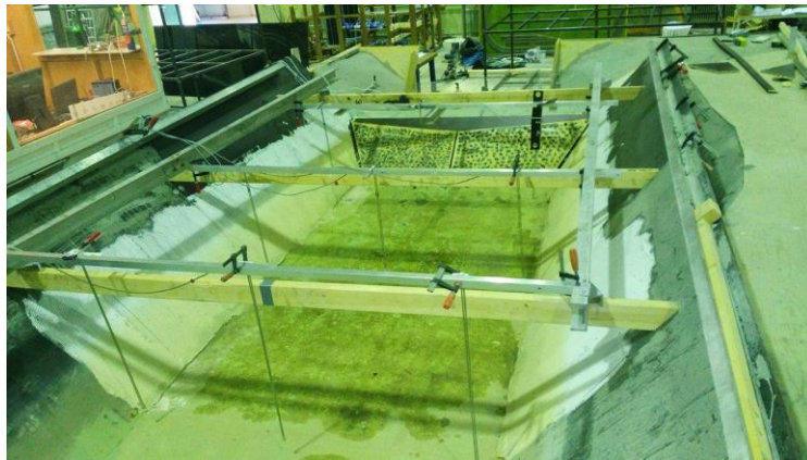
Figure 3.2: picture of the trapezoidal basin with sensors inside and the dam on background.
