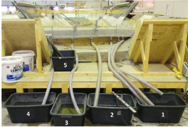
Figure 3.7: picture of the five collecting buckets connected to the plexiglas channel through pipes.
