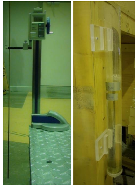
Figure 3.13: water level indicator on the left and piezometer on the right.
