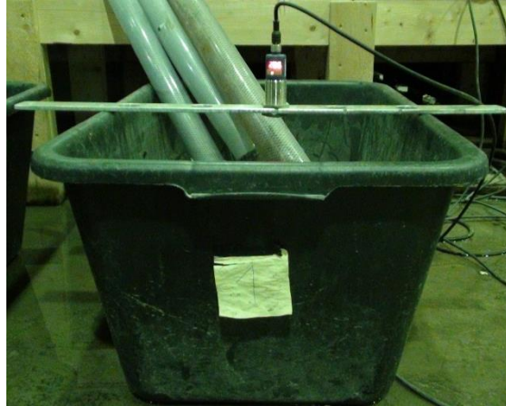
Figure 3.17: ultrasonic sensor used for the evaluation of overtopping volume collected in the buckets.
