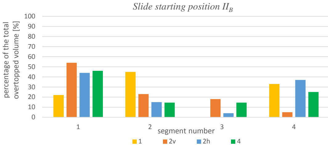
Figure 6.45: the diagram illustrates the percentages of the total overtopped volume measured in different buckets. Each of them is connected to one of the four specific segments of the channel where overtopped water from the dam is funnelled; trials considered are 1.II B , 2v.II B , 2h.II B and 4.II B .
