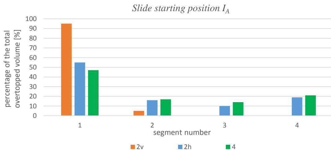
Figure 6.44: the diagram illustrates the percentages of the total overtopped volume measured in different buckets. Each of them is connected to one of the four specific segments of the channel where overtopped water from the dam is funnelled; trials considered are 2v. I_A , 2h. I_A and 4. I_A .
