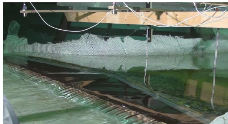
Figure 3.16: ultrasonic sensors above the dam crest during an overtopping event (Mortensen, 2016).
