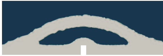
Figure 7.13: Optimal shape for the bypass problem with respect to the energy dissipation functional, with 10 % of the velocity magnitude and \beta = 10.0 .
