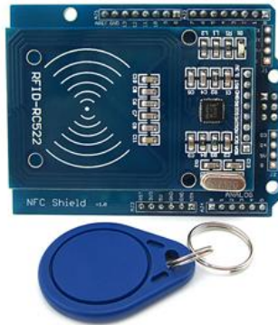
Figure 3.9: RFID keyfob (below) and the RC522 RFID reader
