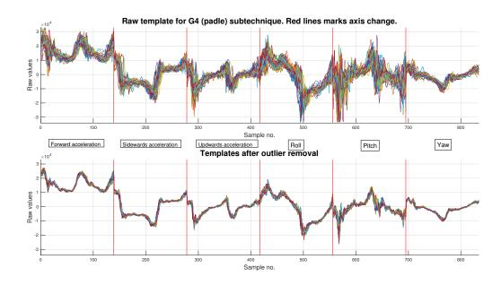
Figure 3.6: Plot illustrating segmented cycles, from the G4 (padle) subtechnique, compiled into overlapping templates. The second subplot illustrate results from outlier removal.
