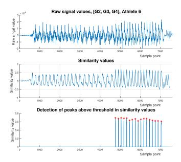
Figure 3.12: Plot illustrating peak detection in similarity values.
