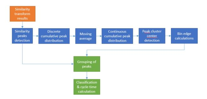
Figure 3.13: Flow diagram illustrating the grouping algorithm.
