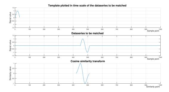
Figure 2.3: Illustration of template matching.
