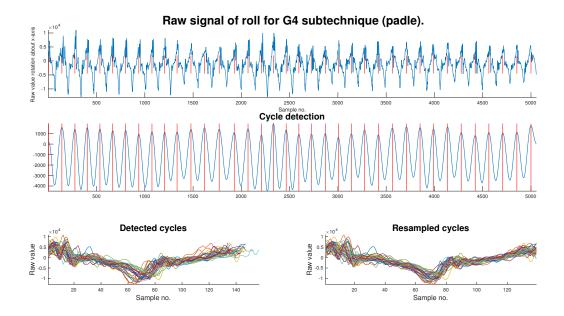
Figure 3.5: Plot illustrating raw data, low pass filtered data with cycle detection, and cycle resampling.
