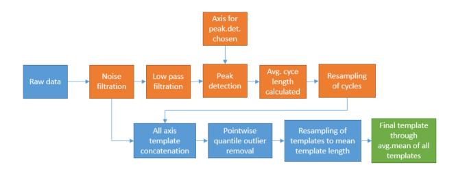
Figure 3.4: Flowdiagram illustrating the template creation algorithm.
