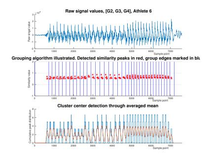
Figure 3.14: Plot illustrating the grouping algorithm.
