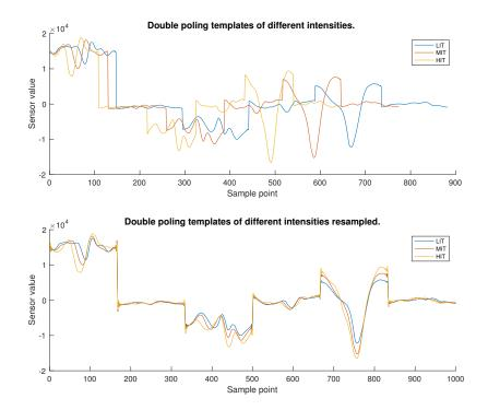
Figure 4.3: Illustration of differing characteristics between different intensities for templates within the same subtechnique
