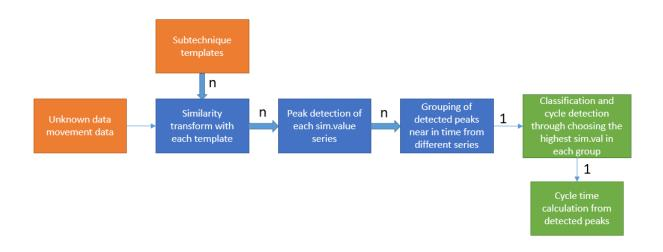
Figure 3.9: Flowdiagram illustrating the template matching algorithm. '*n*' equals number of templates.
