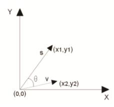
Figure 3.10: Illustration of the cosine similarity transform, with  $\theta$  being the measure of similarity between the vectors *V* and *S*.
