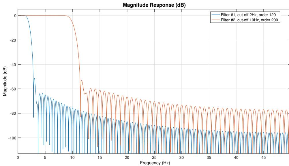
Figure 3.8: Frequency response of the low-pass filters designed and used in this study.
