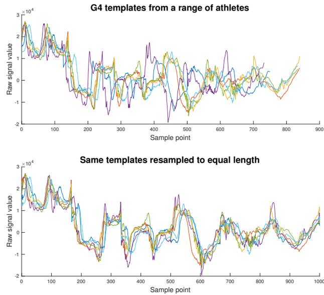
Figure 3.15: Plot showing the effects of resampling templates of the same subtechnique from different athletes to equal length.
