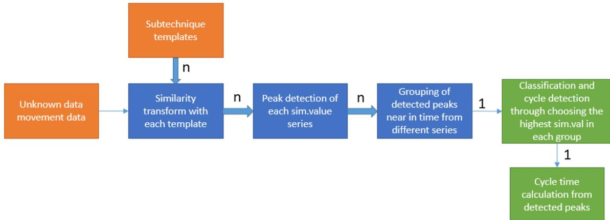
Figure 3.9: Flowdiagram illustrating the template matching algorithm. 'n' equals number of templates.
