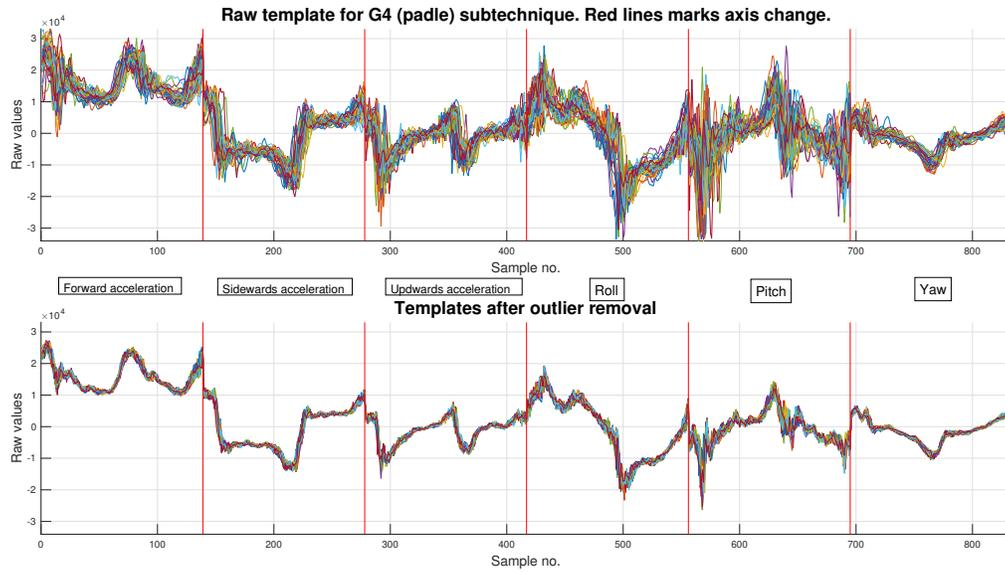
Figure 3.6: Plot illustrating segmented cycles, from the G4 (paddle) subtechnique, compiled into overlapping templates. The second subplot illustrate results from outlier removal.
