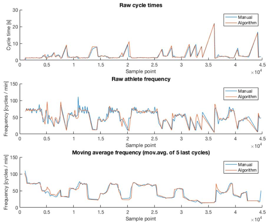
Figure 4.8: Results of cycle time and frequency comparison between manually marked and algorithm produced cycles.
