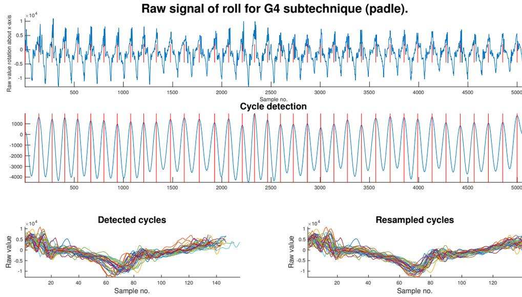
Figure 3.5: Plot illustrating raw data, low pass filtered data with cycle detection, and cycle resampling.
