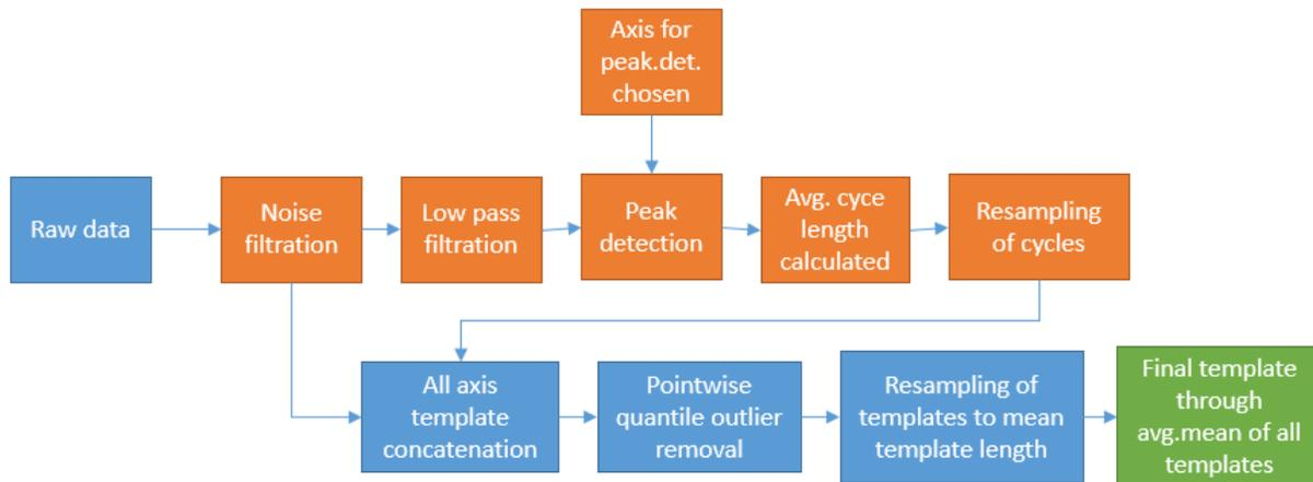
Figure 3.4: Flowdiagram illustrating the template creation algorithm.
