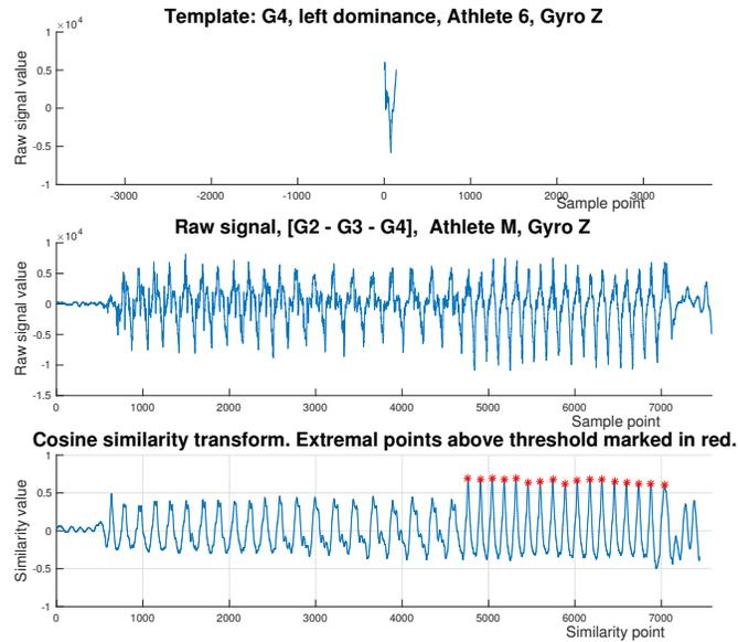
Figure 3.11: Plot illustrating the cosine similarity transform on cross-country skiing data. The upper plot shows the gyro-z axis segment of the template, plotted in the scale of the data for context illustration. The lower data shows the results of the similarity transform, with peaks above threshold marked in red.
