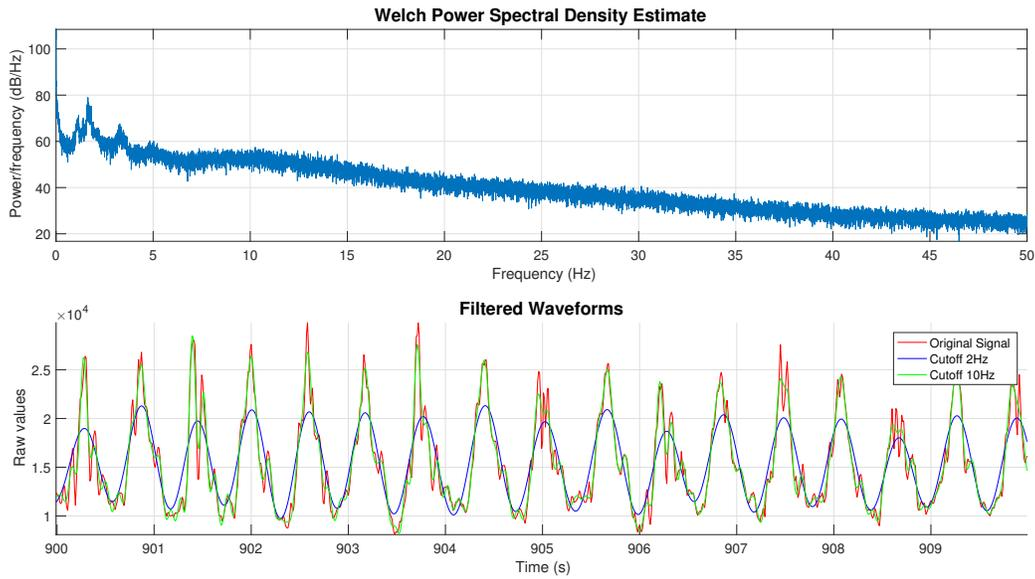
Figure 3.7: Plot illustrating the power spectral density of raw IMU cross-country data and the effects of filtering. The PSD is calculated using Welch’s method.
