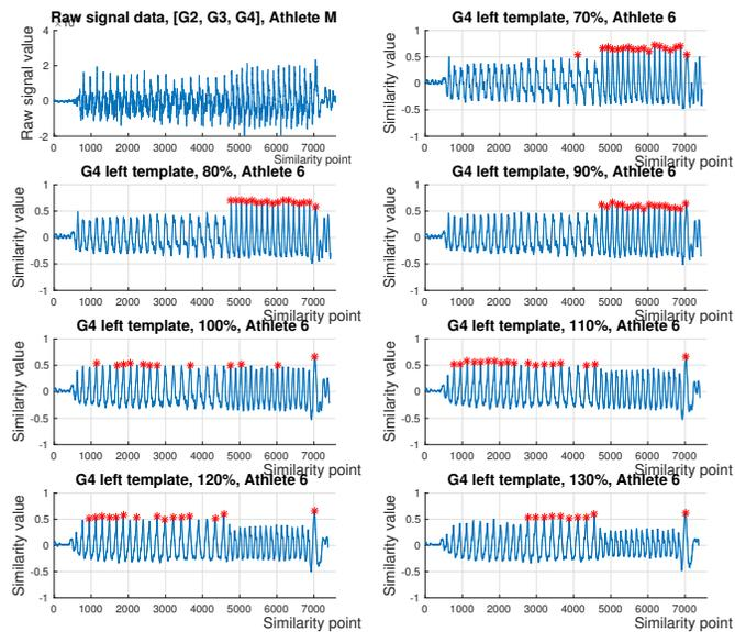
Figure 3.16: Plot showing the effects of using resampled versions of the same template in the similarity transform.
