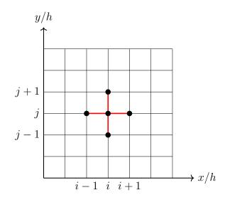
Figure 5.1: Illustration of a two dimensional finite difference numerical scheme.
