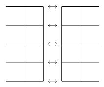
Figure 5.9: Illustration of mesh alignment at an interface between two materials, thus allowing a discontinuous transition.
