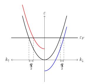
Figure 2.3: Illustration of the splitting of electron bands with opposite spins in the presence of an exchange field.
