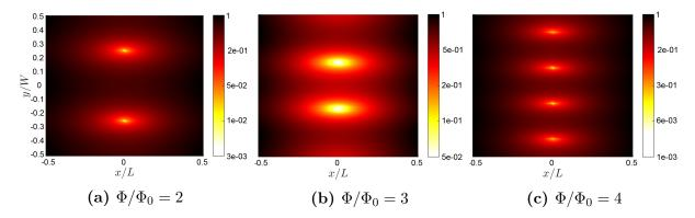
Figure 6.2: The pair correlation for a wide Josephson junction with external flux. The width is  $W = 8\xi$  and the length is  $L = 2\xi$ . The pair corelation function is normalized with respect to its value at the interface to the superconductors.
