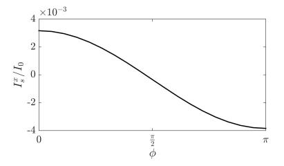
Figure 6.18: Phase dependence of the *x*-polarized spin current. The other polarizations are identically equal to zero.
