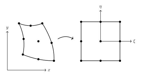
Figure 5.5: Illustration of a transformation to the reference element.
