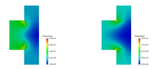
Figure 6.6: The current density in the two geometries, scaled by  $J_0 = \frac{N_0 e D \Delta}{4\hbar}$ .
