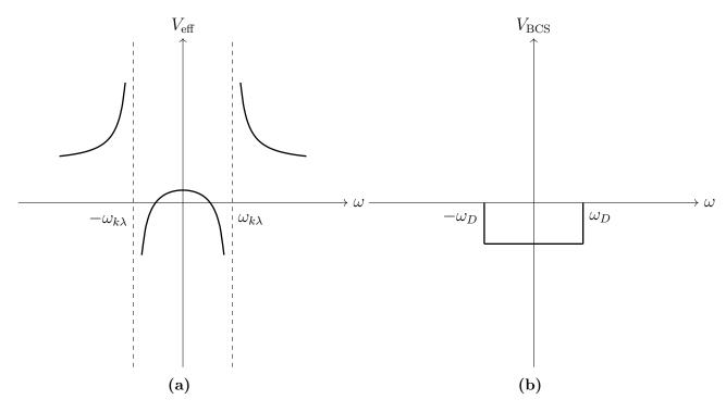
Figure 3.2: The potential used in the development of the microscopic theory of superconductivity. (a) The potential generated by phonon-mediated electronelectron interaction, (b) a simplified potential used in BCS theory.
