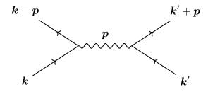
Figure 3.1: Feynman diagram for a phonon-mediated electron-electron interaction.
