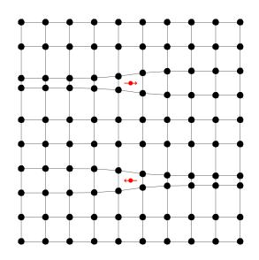
Figure 2.1: Classical illustration of the formation of a Cooper pair. The electrons are marked in red, with arrows indicating their direction of motion.
