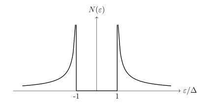
Figure 4.2: Density of states for a bulk superconductor.
