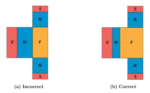
Figure 6.5: Two variations of a T-shaped geometry, one of which displays a poor modeling decision, producing erroneous results.
