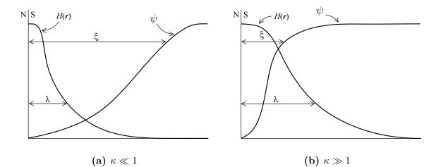
Figure 2.2: Illustration of the behavior of the magnetic field H and the wave function  $\psi$  by a normal metal - superconductor interface for different values of the parameter  $\kappa$ . Adapted from<sup>22</sup>.
