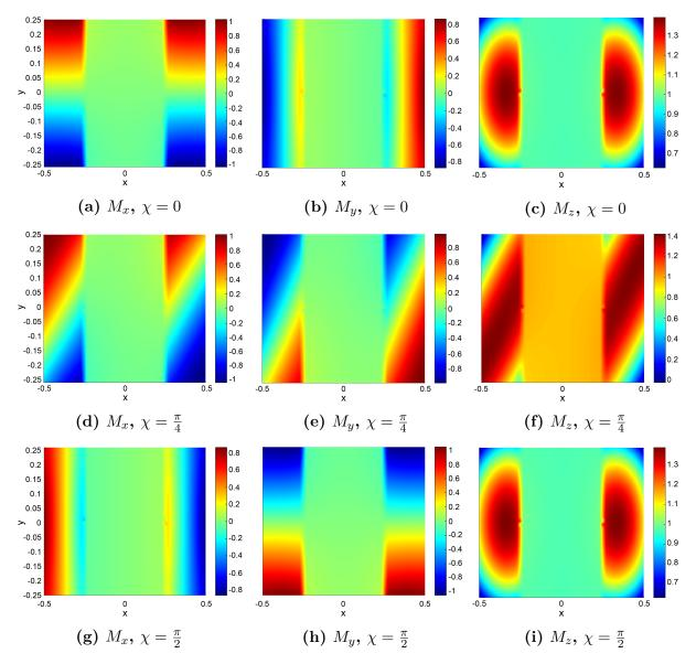
Figure 6.15: The magnetization for different values of the spin-orbit angle  $\chi$ . The results are scaled by  $M_0 = \frac{g\mu_B N_0 \Delta}{8}$ , and the lengths by  $\xi$ .
