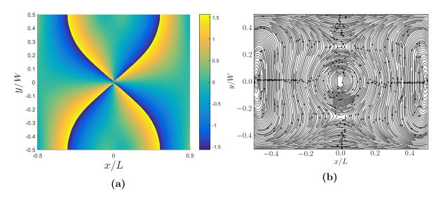
Figure 6.11: Additional information for the configuration where the vortices overlap;  $W = 1.95\xi$ . In (a) is shown the phase of the pair correlation function and in (b) the direction of the current density
