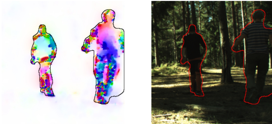
Figure 8.13: The segmentation result for the same experiment as shown in figure 8.9, but with a higher sensitivity parameter for the edge detector ( \eta = 225 ). The shoulder of the person on the right is not as badly described as in the previous experiment, but the curve segments a large region close to the boundary, near the feet, due to some noise in the flow field.
