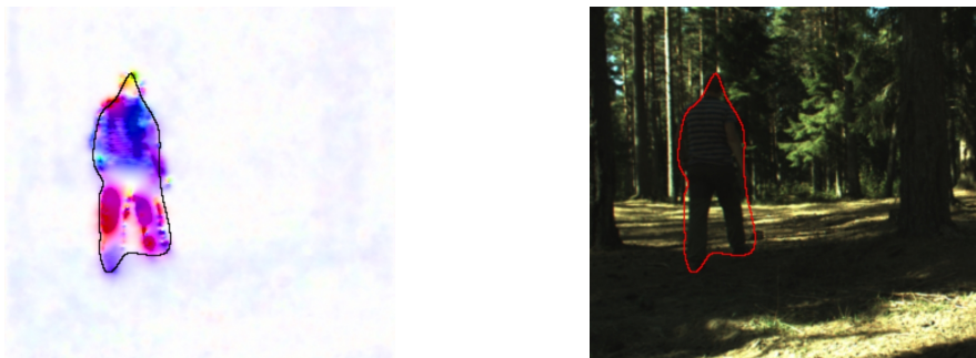
Figure 8.7: The segmentation result of a Horn and Schunck flow field. The level set function is evolved using the same parameters as in the experiment shown in figure 8.6, but with \delta = 100 and \delta' = 2.0 . Two initial level set evolutions was run before commencing with the combined evolution. The result seen above is obtained after one iteration of a 1:50 combined evolution.
