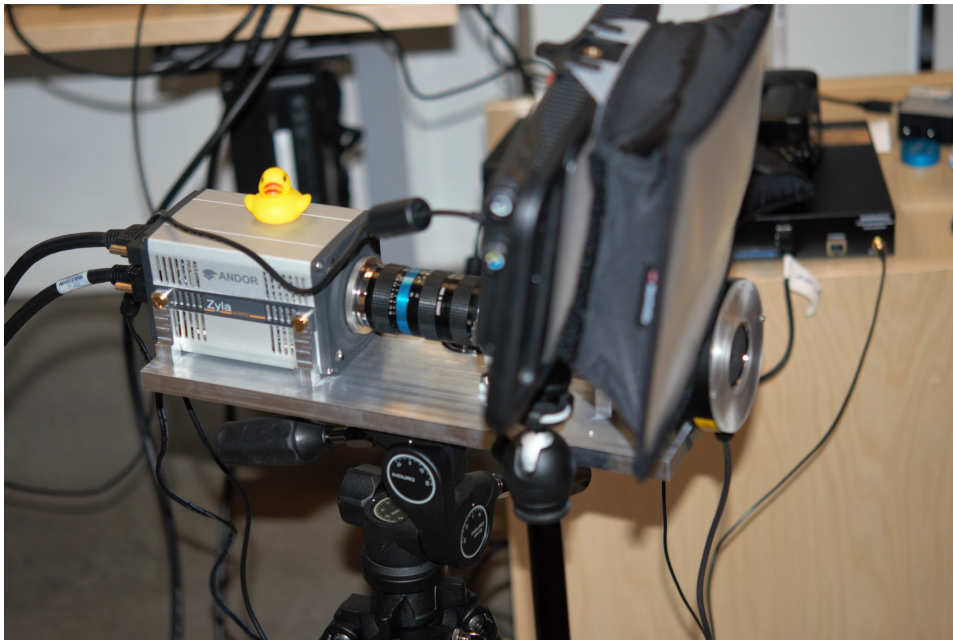
Figure 4.1: The imaging setup used in Oslo on the second trip. Slightly out of focus, in the front, the lamp can be seen. In focus is the camera (with a rubber duck on top), and in the background, the RF-driver and spectrometer can be seen. The main computer is set on the table to the left in the background.
