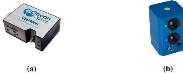
Figure 3.9: Image of (a) the Ocean Optics Spectrometer and (b) integrating sphere used.
