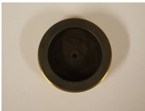
Figure 3.4: Image of the lens coupler for MeVis lenses. This part also serves as a pinhole and holder for a polarising filter.
