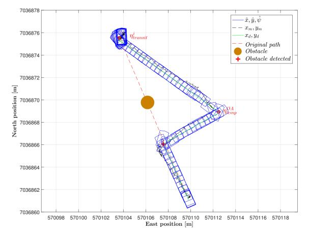
Figure E.1: Estimated, measured and desired ROV position in NE plane
