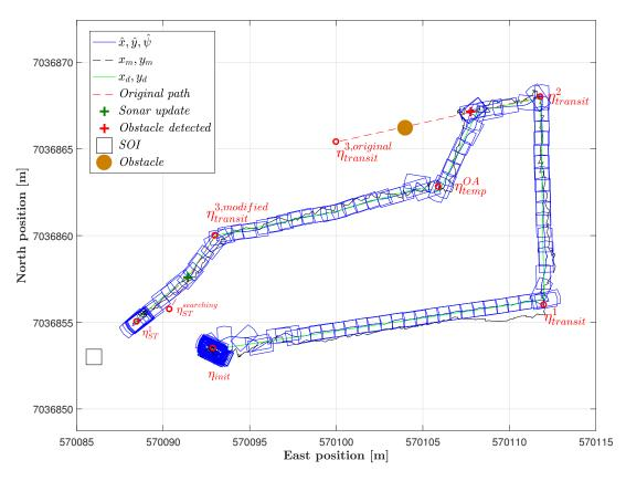
Figure 6.10: Estimated, measured and desired ROV position in NE plane
