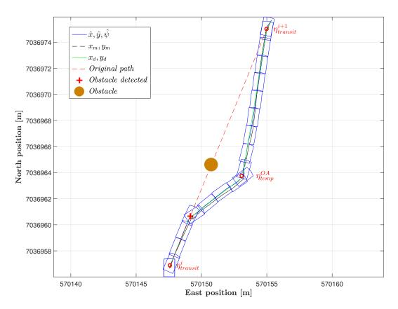
**Figure 5.1:** Estimated, measured and desired ROV position in NE plane,  $\beta = 30^{\circ}$  and d = 5 m
