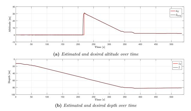
Figure E.11: Estimated and desired ROV altitude and depth over time
