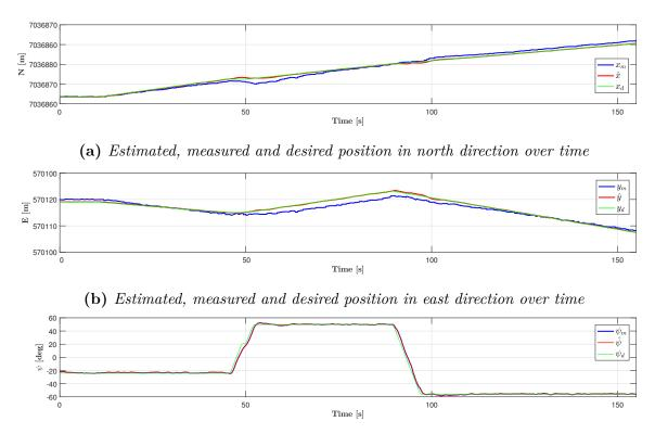
(c) Estimated, measured and desired Heading over time
