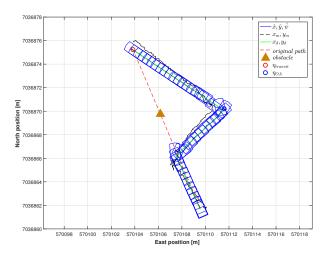
Figure 1. ROV position in xy-plane during collision avoidance.
