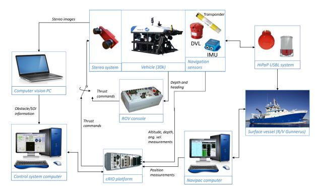
**Figure 4.1:** Information flow between the equipment used for testing the agent architecture. Each block is described in detail in the following sections.
