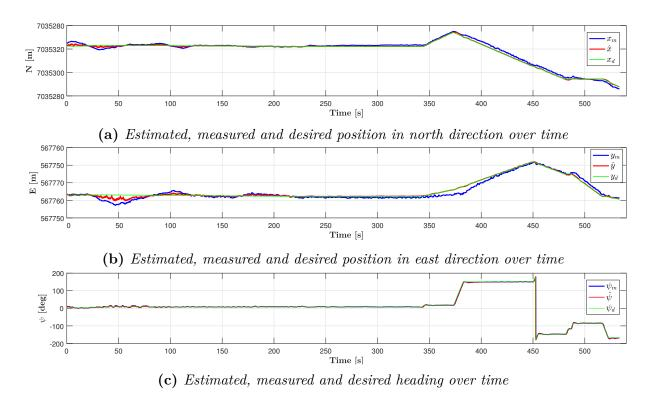
Figure E.10: Estimated, measured and desired ROV position and heading over time
