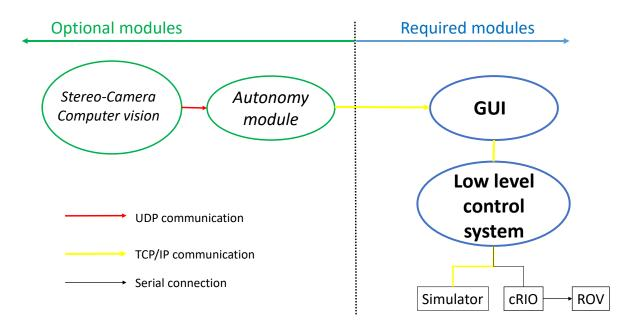
Figure 4.2: Module configuration of (1)-(4).; Basic modules GUI and Control System, connection with optional Autonomy module and its additional module for computer vision. Communication between modules is stated with color coding, and further described in Section 4.1.3 and 4.1.4. Based on Figure 2.4 in [5].
