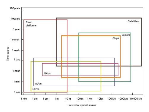
Figure 1.1: Spatial and temporal resolution and coverage of different offshore and over- and underwater platforms [48]
