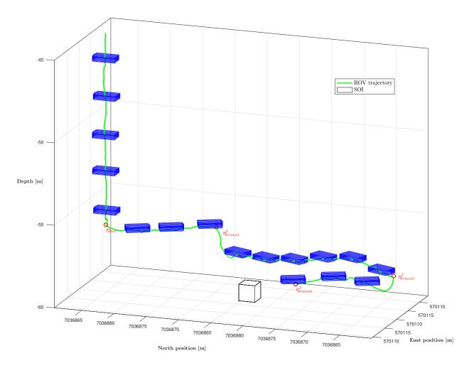
Figure 6.8: 3D illustration of the vehicle during mission control
