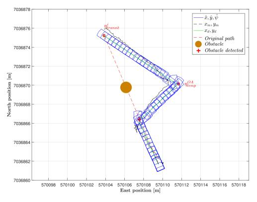
**Figure 6.1:** ROV position in NE plane,  $\beta = 30^{\circ}$  and d = 5 m.
