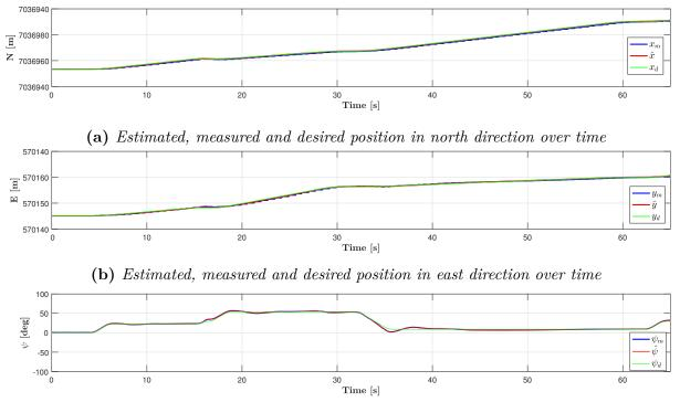
(c) Estimated, measured and desired heading over time
