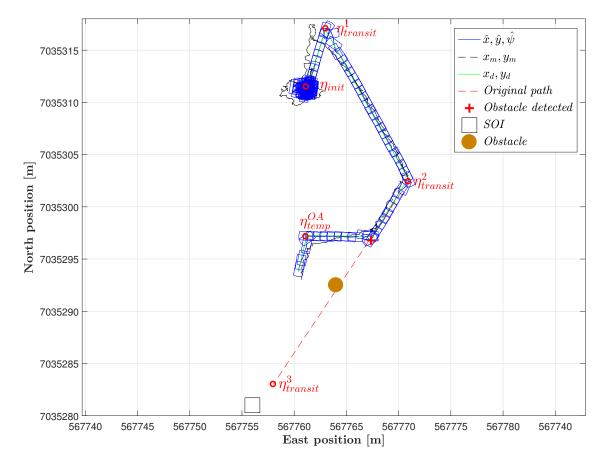
Figure E.9: Estimated, measured and desired ROV position in NE plane
