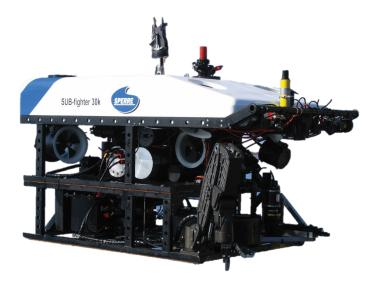
Figure 4.3: ROV SUB-fighter 30k [53] ready for deployment in the Trondheim fjord
