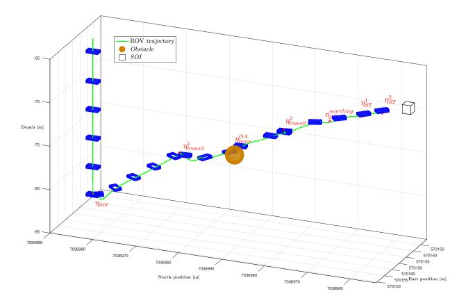
Figure 5.12: 3D illustration of the vehicle during mission control
