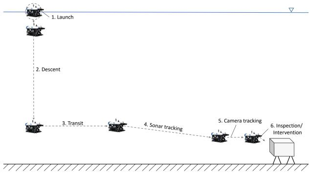
Figure 3.5: Autonomous mission: approach and localization of SOI
