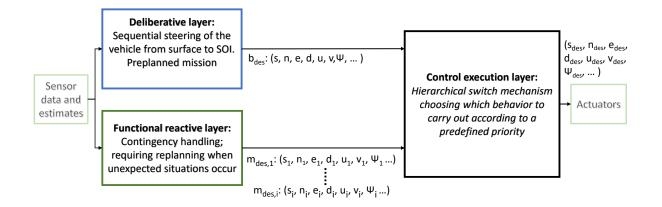
Figure 3.1: Decomposition of the hybrid agent into three layers, based on Figure 3.1. This diagram is specialized for approaching and locating an SOI on the sea bottom. Each layer outputs a behavior in terms of parameters described in Table 3.1.  $m_{des,i}$  are the active reactive behaviors, while  $b_{des}$  is the active deliberative behavior.
