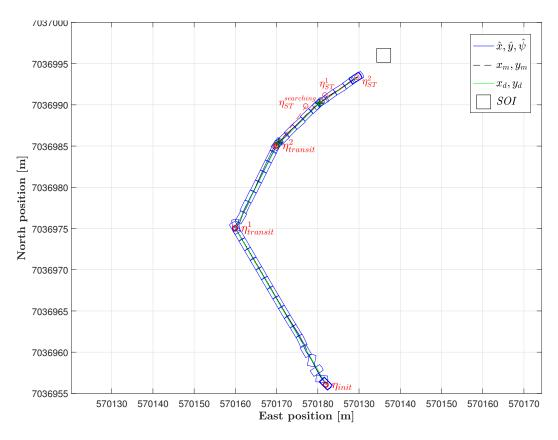
Figure 5.5: Estimated, measured and desired ROV position in NE plane
