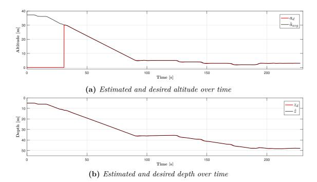
Figure D.3: Estimated and desired ROV altitude and depth over time
