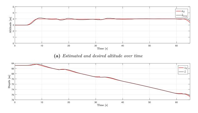
(b) Estimated and desired depth over timeFigure 5.3: Estimated and desired ROV altitude and depth over time
