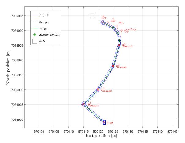
Figure D.1: Estimated, measured and desired ROV position in NE plane
