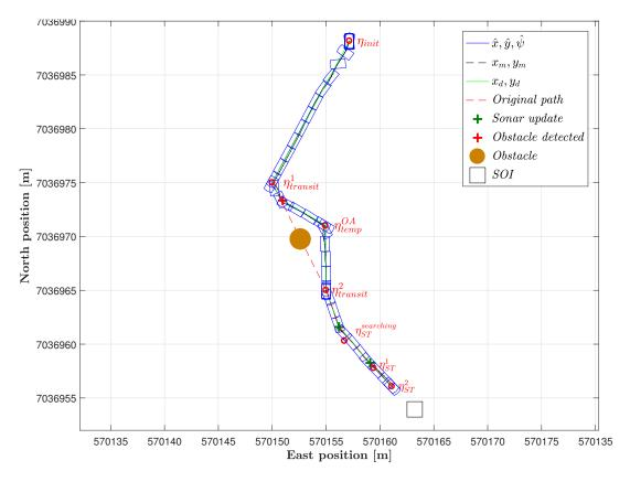
Figure 5.9: Estimated, measured and desired ROV position in NE plane
