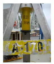
(b) Transponder attached to tripod forming a transponder tower [3]. The tower carries one of four transponders in the LBL network deployed outside TBS in 2013 [3]. The transponders are located 250 and 400 meters away from land.
