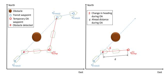
(a) Complete OA during Transit state. The OA state creates a new, temporary waypoint,  $\eta_{temp}^{OA}$ , for the vehicle to avoid the detected obstacle. Reaching this waypoint, the vehicle may return to the desired Transit waypoint.
