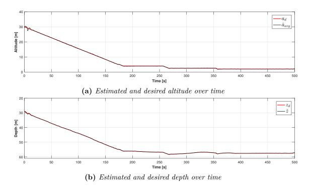
Figure E.7: Estimated and desired ROV altitude and depth over time
