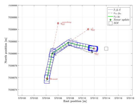
Figure 6.9: Estimated, measured and desired ROV position in NE plane
