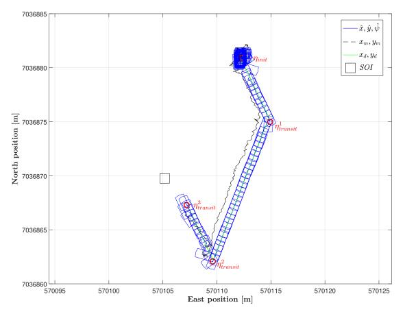
Figure 6.5: Estimated, measured and desired ROV position in NE plane
