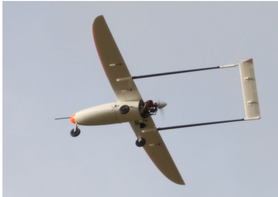
Figure 3.13: Penguin B UAV in flight. Photo: Jakob M. Hansen.
