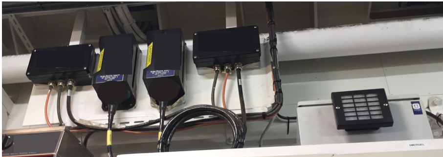
(c) Locations of sensors. Sensor cabinet (bottom right) located close to the onboard VRUs (top left).
