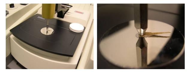
**Figure 2.** A small wood piece from the wood sample was pressed onto the diamond crystal in the ATR accessory connected to the FTIR spectrometer. In the close-up photo to the right, the lower steel pin is only a reflection of the above steel pin in the polished mirror-like sample plate.
