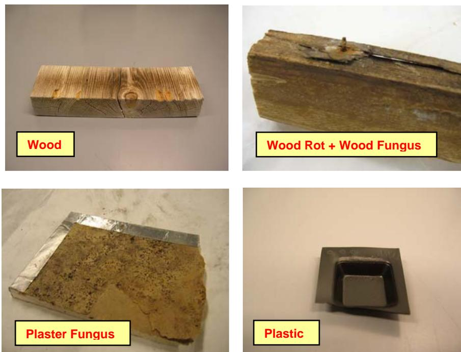
**Figure 1.** Wood, Wood Rot, Wood Fungus, Plaster Fungus and Plastic samples. Small pieces are cut from the samples for use in the FTIR investigations, except the Plastic sample which is used directly.
