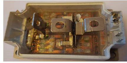
(a) Internal layout of CAS300M12BM2 (Cree).
