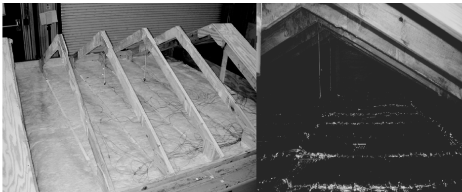
Fig.5. The tested attic construction [left] with only the fibreglass batts between wooden beams and without roof shelter and [right] a view in the attic construction when the GFPs with the attic radiant barrier are installed (Yarbrough et al. 2007).
