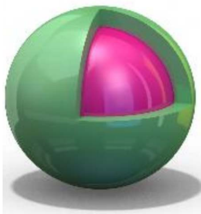
Figure 3 Model of a microencapsulated PCM with a wax core and polymeric shell (Phase energy [84]).
