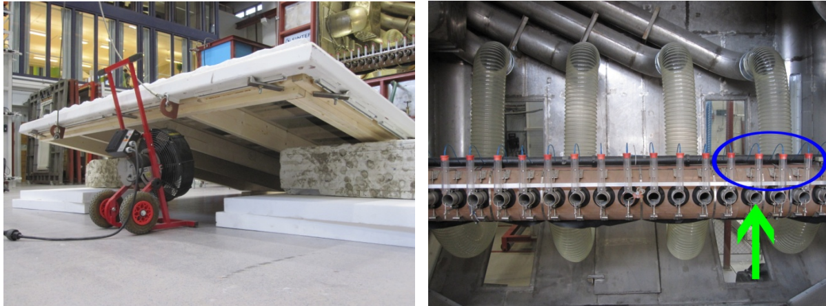
Fig. 5: Drying of BIPV sample roof with fan heater between test phases (left), and the boom inside the RAWI box which delivers wind-driven rain across the sample area (right). Water runs from the blue tubes on top (blue ellipse), drips down the transparent vertical cylinders (blue ellipse), and is blown onto the sample area as it hits the air stream that blows out of the air tubes (green arrow).
