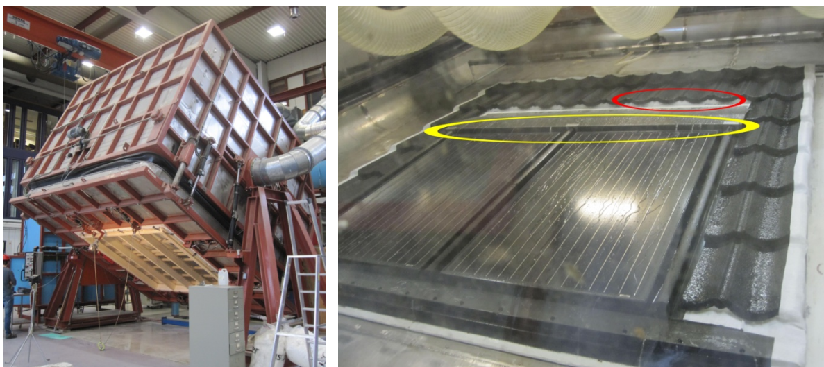
Fig. 4: Visual inspection of BIPV sample roof from below the inclined RAWI box (left) and sample roof inside the RAWI box during testing, viewed from outside the box through a window (right). The coloured ellipses denote leakage points.
