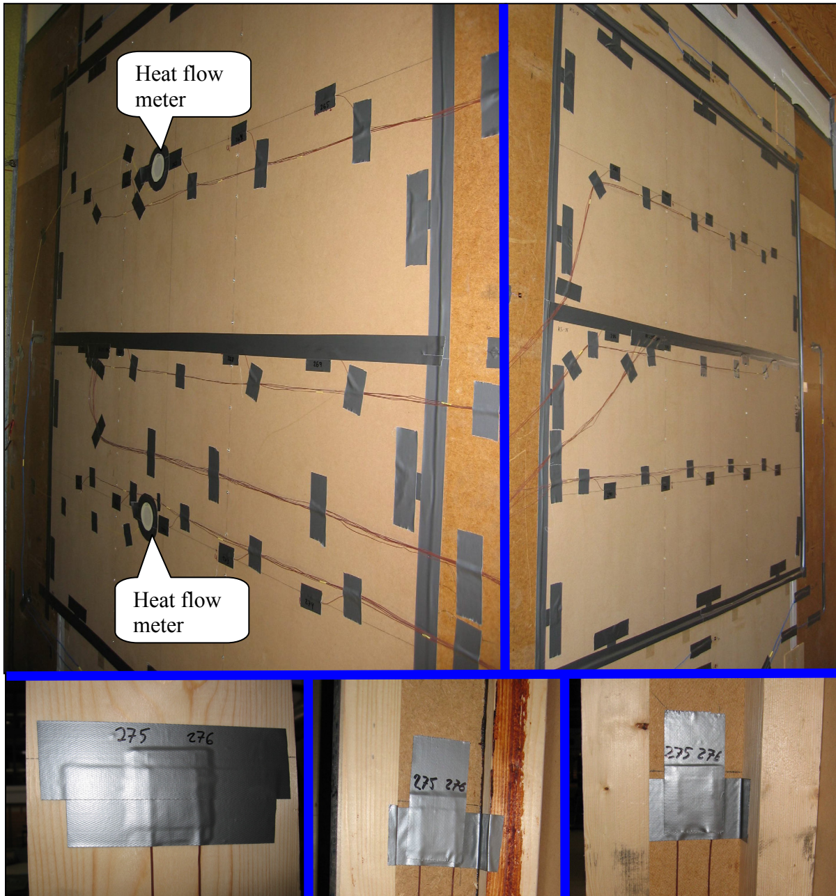
Figure 6 Placement of thermocouples and heat flow meters on wall and studs. Upper left: Hot side, Upper right: Cold side. Lower left: 36 mm stud, Lower middle: I-stud, Lower right: U-stud.
