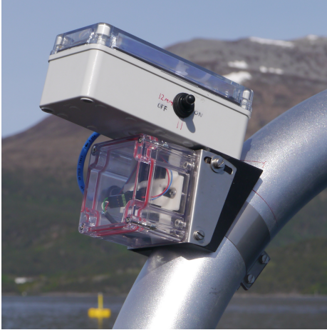
Figure 3.3: Attitude measurement system (AMS) 1.0 mounted to the center pipe of the spreader.
