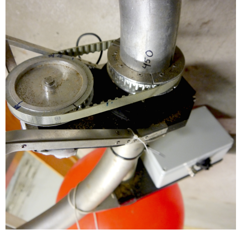
Figure 3.4: Attitude measurement system (AMS) 2.0 mounted to the base of the spreader with an additional rotary encoder.
