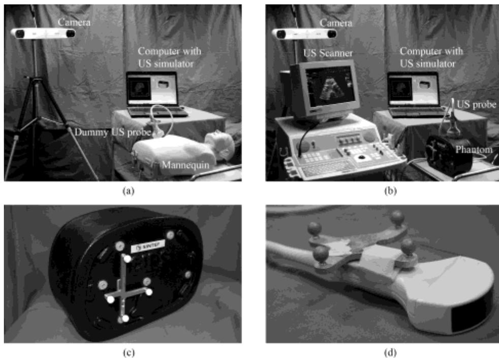
**Figure 2:** Ultrasound simulator (a) and laboratory setup for the evaluation of the simulator (b). The camera tracks the position of the probe relative to the phantom. A simulated image corresponding to the image on the display of the ultrasound scanner is generated based on this position. The phantom with fiducials and positioning frame is shown close up in (c), and the ultrasound probe with positioning frame in (d).
