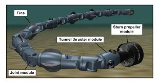
Fig. 1: Concept illustration of an underwater swimming manipulator
