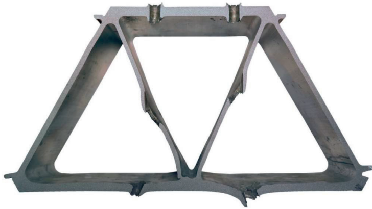
Figure 6: Cross section of an AA6005-T6 panel that was struck without sand. Left: v_i = 618.9 m/s and v_r = 386.3 m/s. Right: v_i = 534.9 m/s and v_r = 292.6 m/s.
