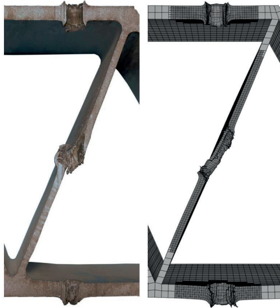
Figure 23: Pictures of an experiment and a simulation of a sand-filled panel to show the qualitative similarities. Left: experiment ( v_i = 910.5 m/s and v_r = 485.4 m/s). Right: simulation ( v_i = 900.0 m/s and v_r = 431.0 m/s).
