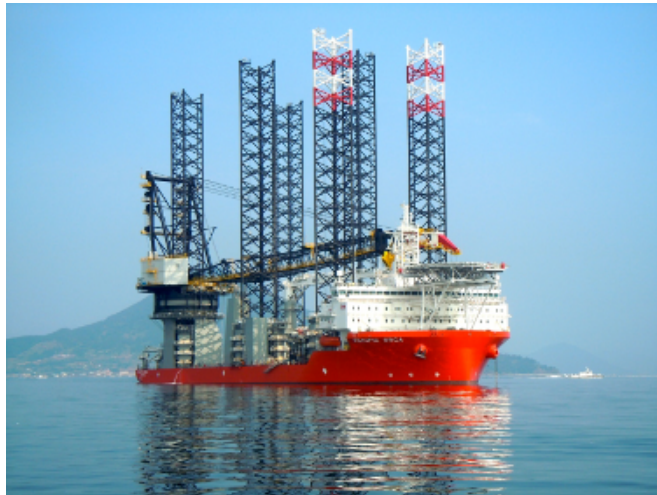
Figure 5: Wind turbine installation jack-up vessel Pacific Orca [32]
