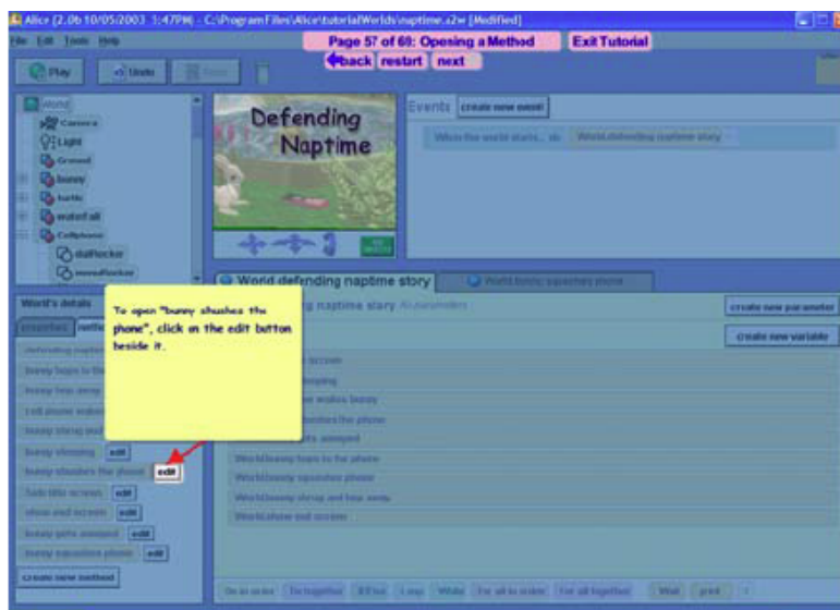
Figure 3.1: An example of highlighting relevant UI elements with Stencils through holes in the colored layer. Tutorial information is added with the yellow sticky note. Image source: [KP05]
