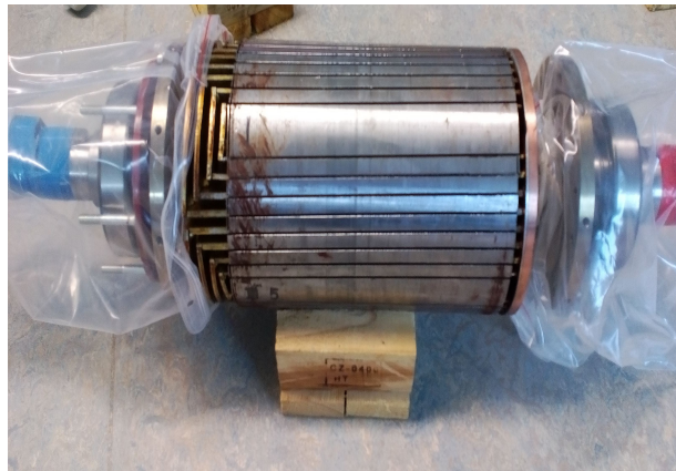
Figure 2.3: Skewed Nested cage rotor.
