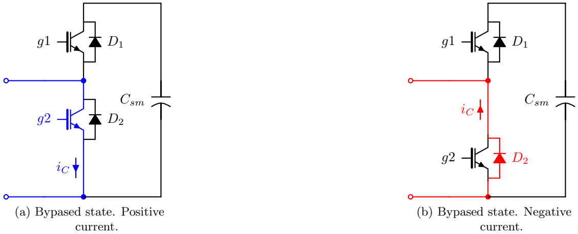
Figure 4.4: Bypassed states of submodule operation. Where blue is for current flowing in the right direction and red is for current flowing in opposite direction.
