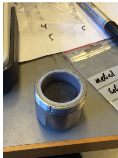
Figure 5.4.2: Slag in powder form after one round of crushing.
