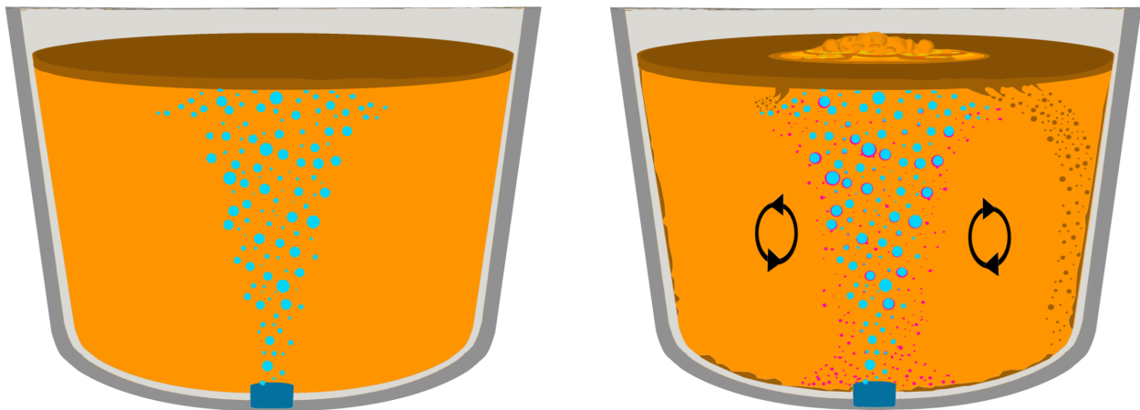
(a) Enriched air is poured from the bottom through a nozzle creating a bubble column. The brown layer represents the slag.
