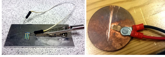
Figure A.1: The sample holders used for electroluminescence. The picture to the left is a prototype with a back contact of aluminum, and the picture to the right is the final version made of copper and wires attached to both front and back contact.
