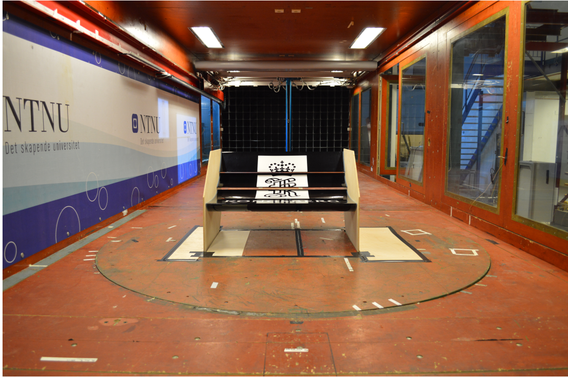
FIGURE 3.8: The three element wing test piece mounted on the force balance in the NTNU wind tunnel.
