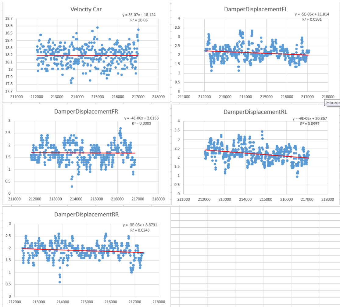
FIGURE A.2: Optical sensor measurements of car velocity along with damper displacement measurements for the front left (FL), front right (FR), rear left (RL) and rear right (RR) wheels, as viewed from the driver. Run 2.
