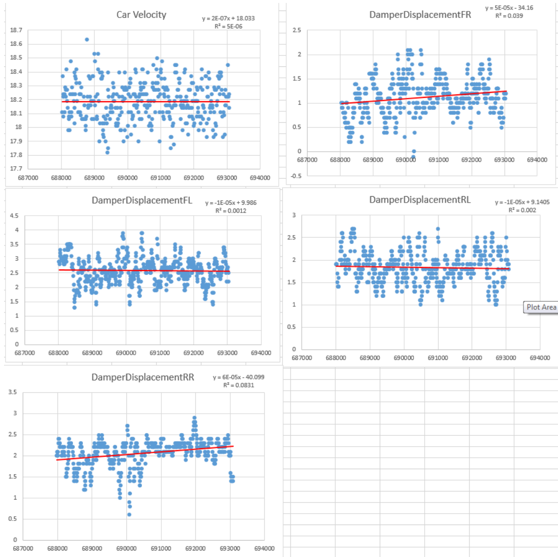
FIGURE A.5: Optical sensor measurements of car velocity along with damper displacement measurements for the front left (FL), front right (FR), rear left (RL) and rear right (RR) wheels, as viewed from the driver. Run 5.
