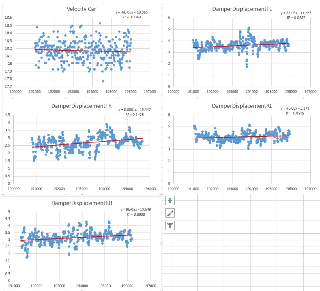
FIGURE A.1: Optical sensor measurements of car velocity along with damper displacement measurements for the front left (FL), front right (FR), rear left (RL) and rear right (RR) wheels, as viewed from the driver. Run 1.
